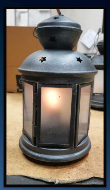
I built a stand which held the light that was soldered to a battery clip, flicker chip & switch. The switch was glued into a hole drilled on the top of the lamp for actors to operate.
